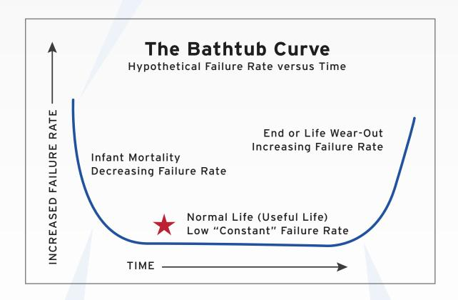
Move down the curve by signature and cycle testing.
