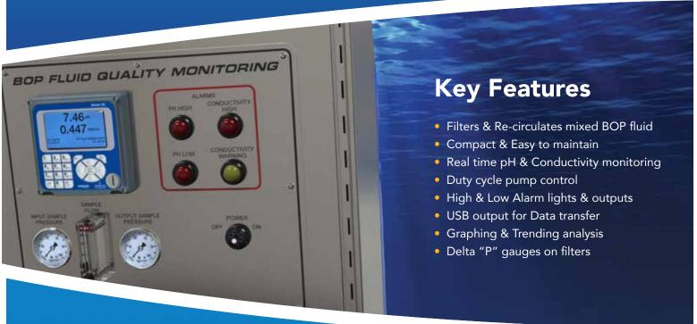
BOP Mixed fluid is subject to contamination from particles, chemicals and microbial growth. The Subsea Company's system recirculates the mixed fluid through a 5 micron filter, exposes the fluid to UV light then passes the fluid though a 1 micron filter. The conditioned fluid's pH and conductivity are then measured providing indications of the BOP mixed fluid quality for event identification and trending analysis.
